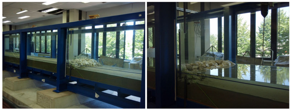
Fig. 1 Physical model of movable-bed and breakwater in the flume ( left panel ) and with water inside ( right panel )
