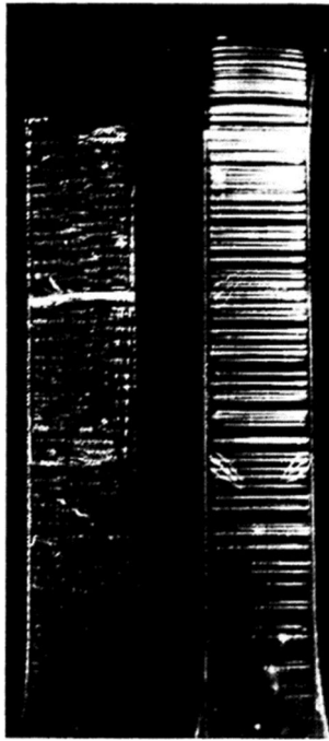
Fig. 16 Craze formation in polystyrene [8]
