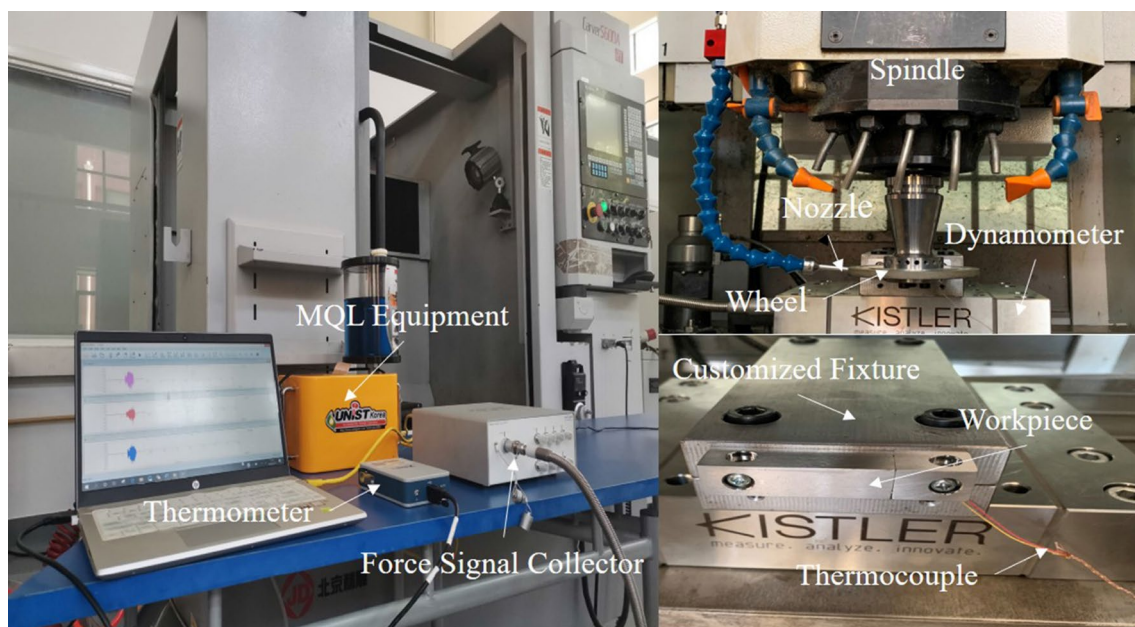
Fig. 6 Grinding experimental setup
