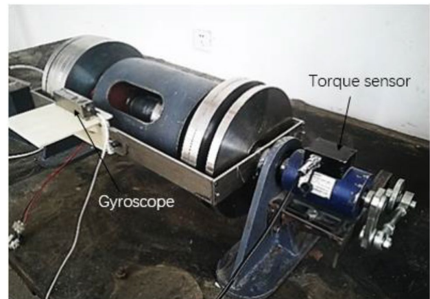
Fig. 5 Prototype of power generation device
