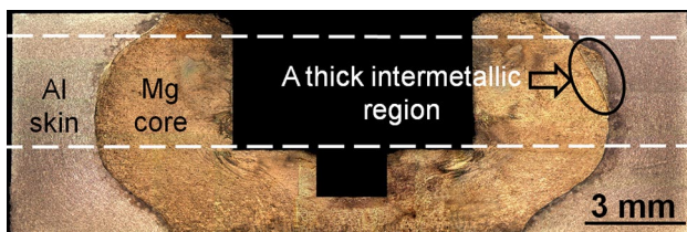
Fig. 5 Optical microscopic image of a forged bimetallic blank
