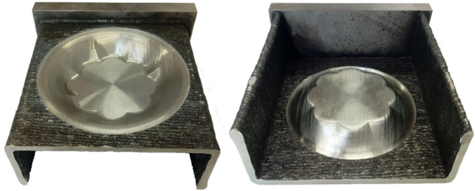
Fig. 11 Top and bottom view of a truncated eight lobe conical shape produced by a hybrid processing route comprising metal deposition by WAAM, milling and incremental forming
