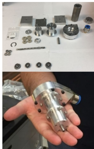
Fig. 8 Turbo-spindle components including assembly tools and fixtures (top), and assembled prototype (bottom)
