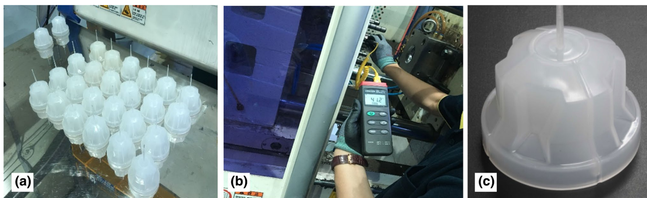
Fig. 11 The molding shots (a), mold temperature measurement device (b), and molded part with good quality (c)
