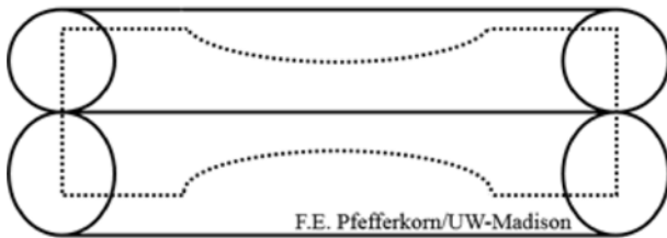
Fig. 6 Top view of deposition passes with material remaining after machining overlaid (not to scale)
