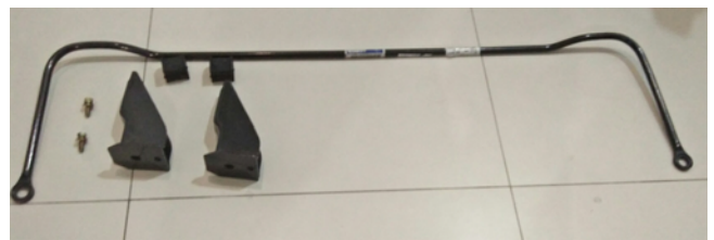
Fig. 3 Automotive anti-roll bar and its components
