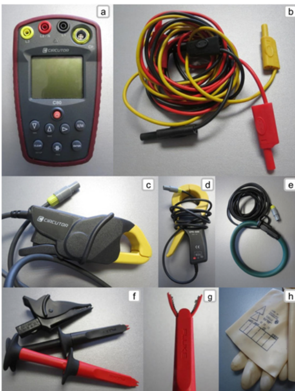
Fig. 1 Measurement equipment: (a) Energy monitoring device, (b) Voltage wires, (c)-(e) Clamps, (f), (g) Crocodile clamps (for voltage wires), (h) Security gloves
