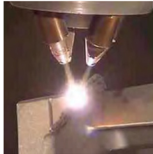
The LENS process, courtesy of Optomec
