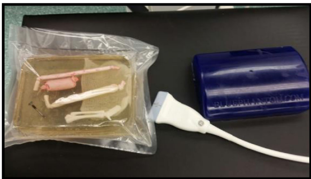
Fig. 1 Homemade ballistic gelatin phantom (left) with embedded screw, gauze, \frac{1}{8} " \frac{1}{4} " and \frac{1}{2} " penrose drain filled with water, miniature plastic skeleton forearm, and hand. Commercial-Grade Blue Phantom™ (right) branched 2-vessel model. Linekar transducer 12 L (middle)
