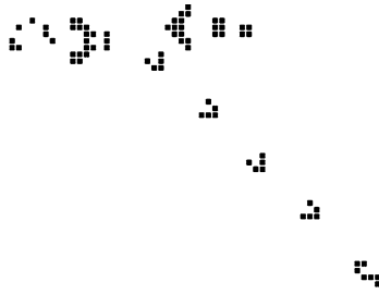
Fig. 3 Gliders in a Game of Life simulation. In this grid, cells are either white or black , and the state of a cell in line n + 1 is determined by the state of the parent cells ( white/black ) in line n and its two neighbors according to a rule. Gliders are these patterns of black dots extended through several lines that are conserved as such along many steps of the simulation, therefore that seem to “move” (translate while rotating) regularly through the grid towards the bottom right , even though the cellular automaton only determines the state of cells in each line
