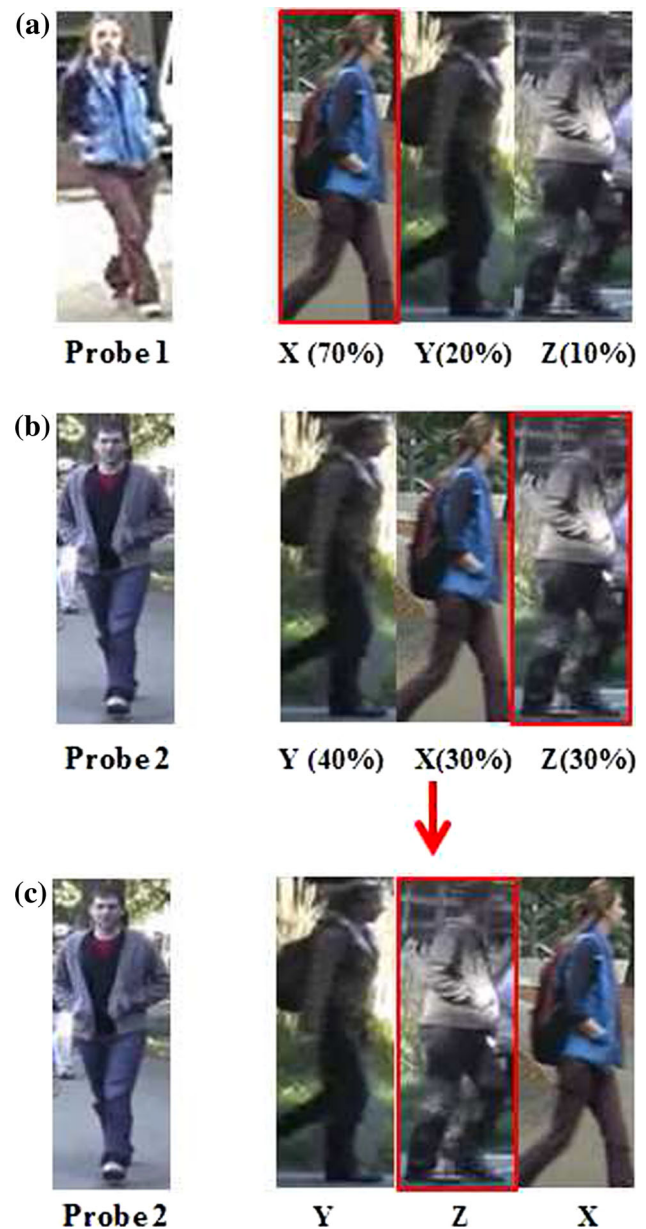
Fig. 2 An example of re-ranking: a Probe image 1 and its ranked list; b Probe image 2 and its ranked list; c Probe image 2 and its re-ranked list based on ranked list (a)
