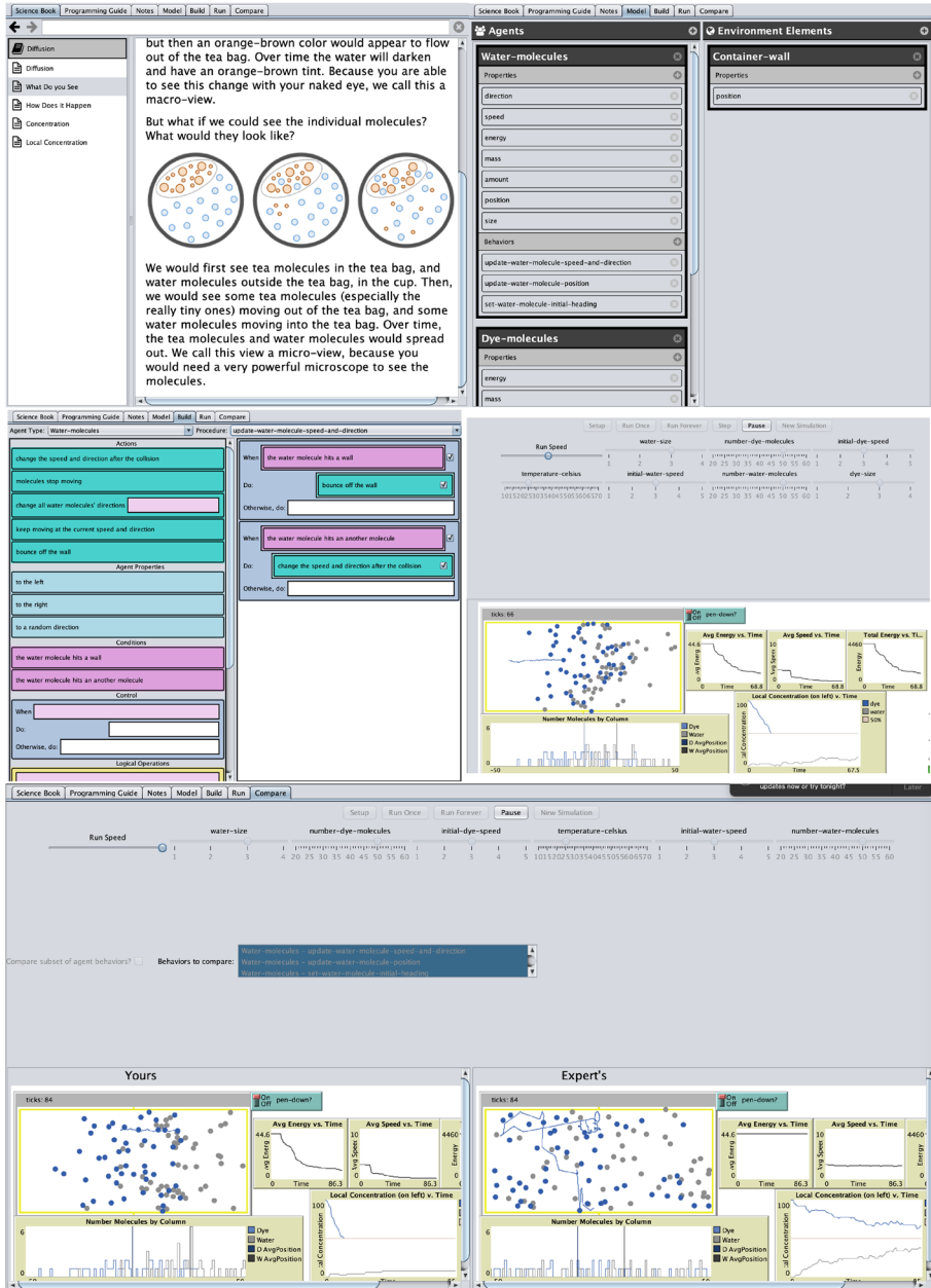
Fig. 1 The graphical user interface and learning activities of CTSiM. The top pane illustrates the Resources window; The middle pane illustrates the Solution Construction (model-building) window; and the bottom pane shows the Solution Assessment (study and compare model behaviors) window
