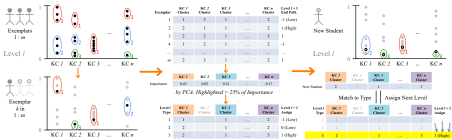
Fig. 8 The data-driven proficiency profiler. (Left) At each level interval, exemplar KC scores are clustered, and exemplars are assigned a cluster for each KC Score. (Center) KCs that make up 25 % of importance in the current level are used to assign exemplars to types. (Right) New student scores are assigned to clusters, and compared to existing types to determine next level path
