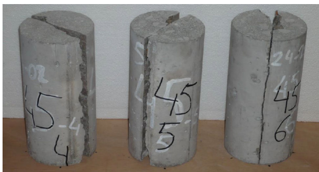
Fig. 6 Specimens after the BTS test
