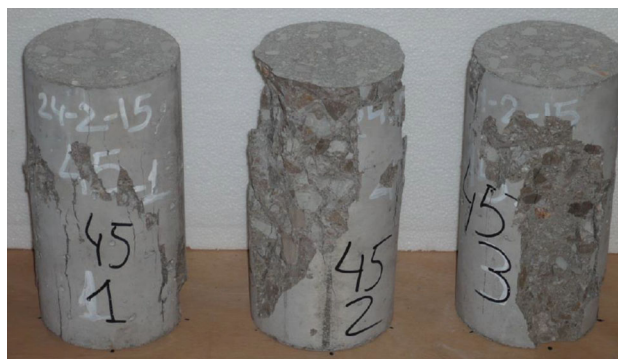
Fig. 4 Specimens after the UCS test
