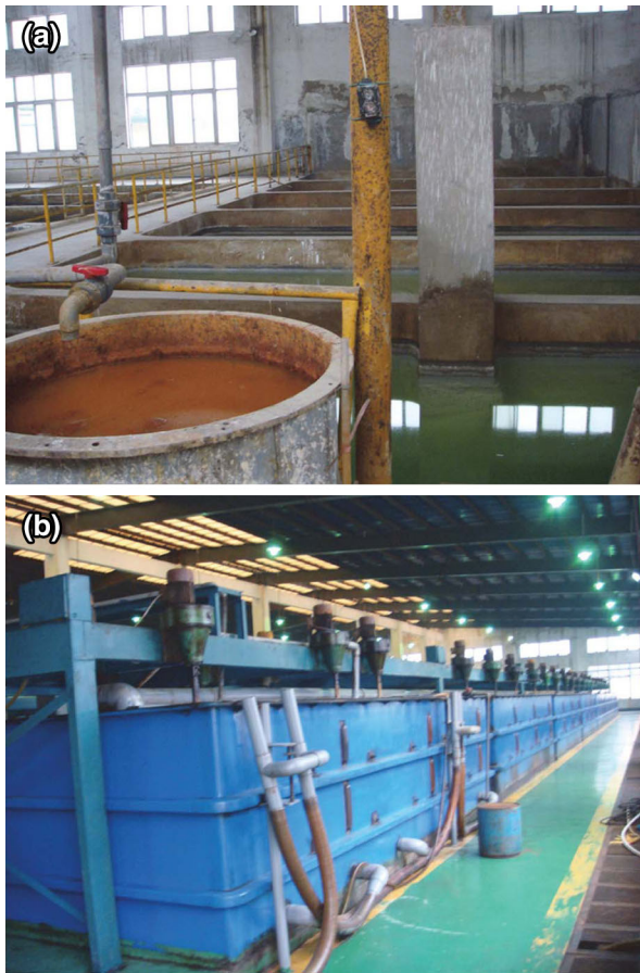
Fig. 8—Photographs of solvent extraction process for mutual separation of rare earths in a plant of China. (Courtesy of Prof. Atsushi Shibayama of Akita University).
