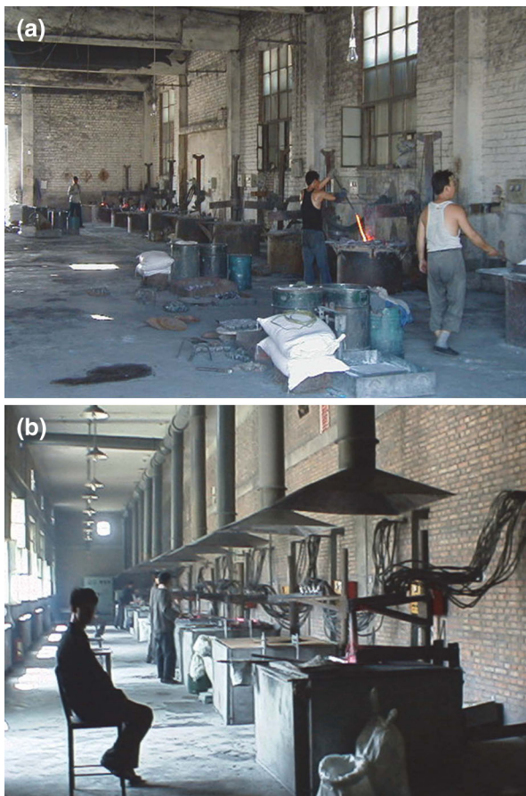
Fig. 6—Photographs of molten salt electrolysis process for producing rare earth metals and alloys in a plant of China. (Courtesy of Dr. Eiji Nakamura of Santoku Co. Ltd.).
