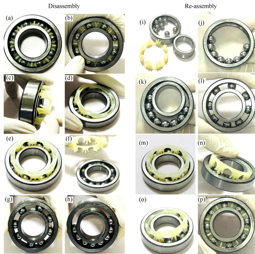
Fig. 2 Photographic illustration of disassembly (a) to (h) and reassembly (i) to (p) of a test ball bearing.
