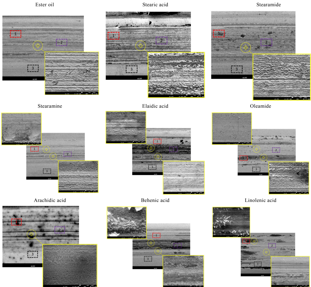
Fig. 16 SEM micrographs of the worn surfaces at 160 \times and 3,000 \times magnification: the numbers show the positions identified for EDX analysis.
