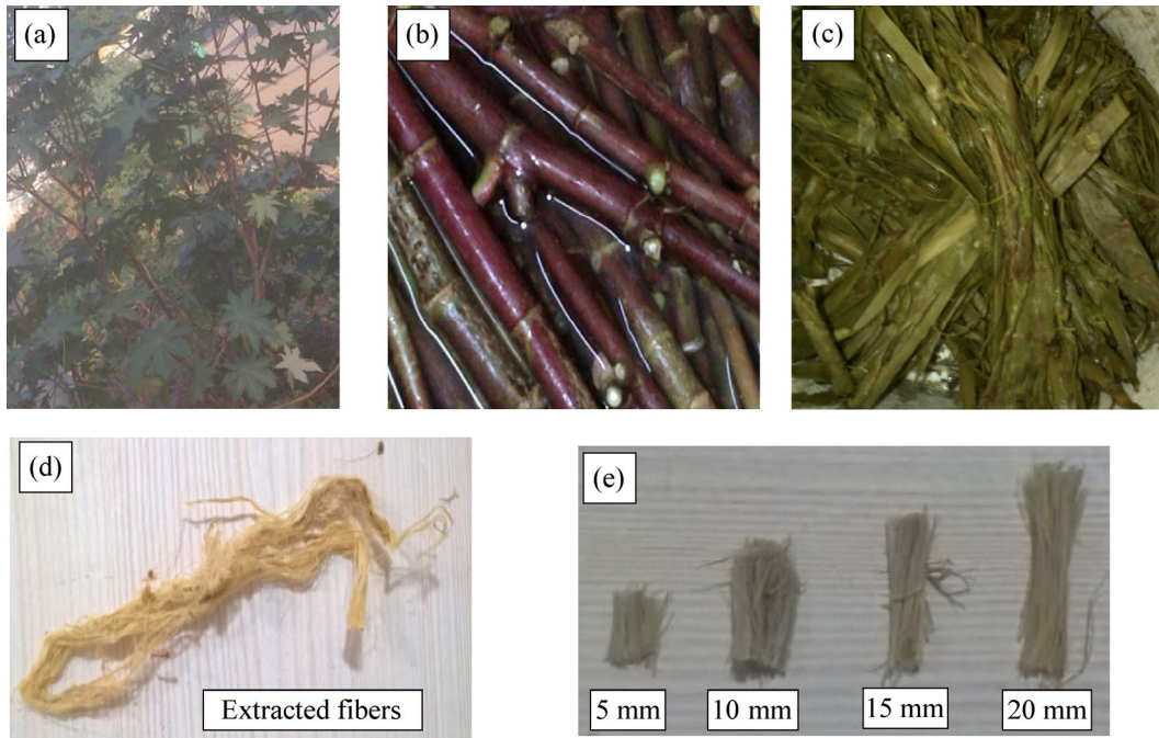
Fig. 1 Fiber extraction procedure. (a) Castor oil plant, (b) stems immersed in water, (c) stems after immersion, (d) extracted fibers, and (e) chopped fibers.
