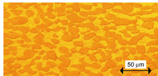
Fig. 1 DSS microstructure in the annealed condition.
