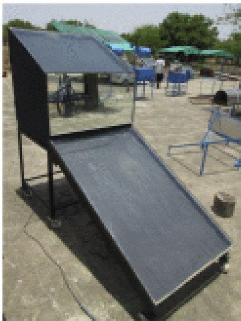
Fig. 7 Photograph of the thermal storage based solar dryer [19]
