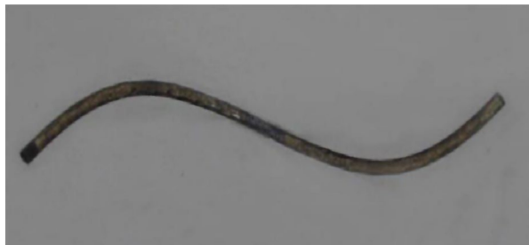
Fig. 12 Tube forming using laser. [Reprinted from [156] with permission from Elsevier]
