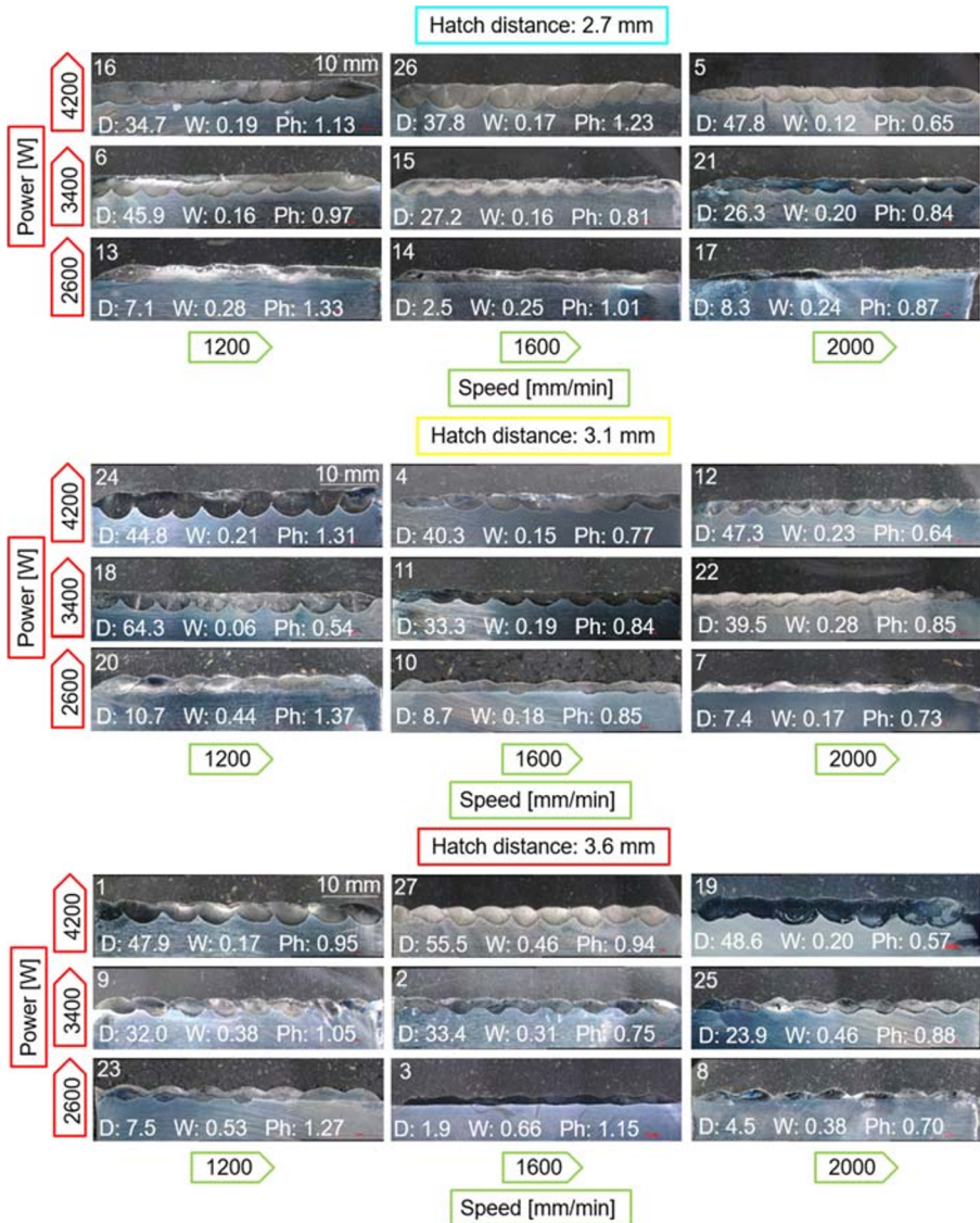
Fig. 5 Cross sections and geometric parameters of obtained coatings (D = dilution [%], W = waviness [mm] and Ph = Peak height [mm])
