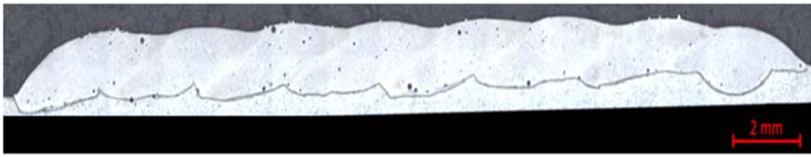
Fig. 8 Cross section of the coating obtained on the validation test
