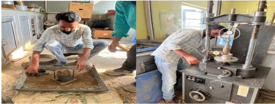
(c) Compaction Test
