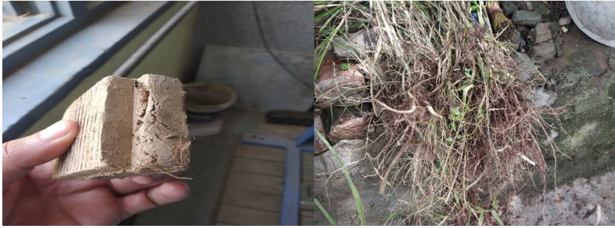
(a). Sheared soil sample failure with the application of root
