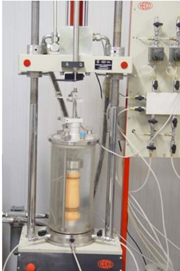
Fig. 4 Triaxial test apparatus setup
