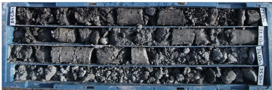
Fig. 5 Mud, sand, and gravel units in the YTSK-1 borehole at the tunnel route (Fugro Sial, 2019a)
