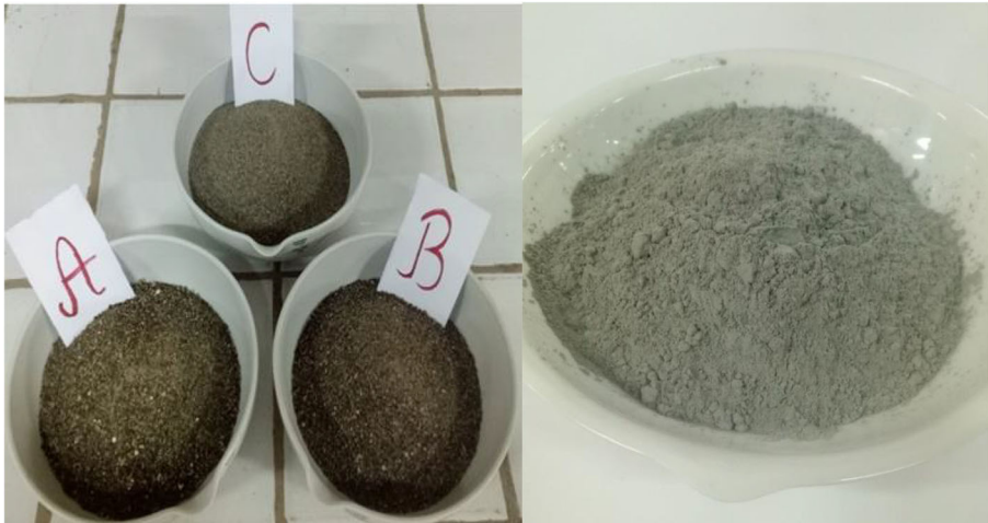
Fig. 1 Granular materials considered in this study. a Categories of Chlef sand. b Fly ash
