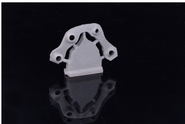
Fig. 26 Rigid impression splint after milling in pre-sintered cobalt-chrome metal
