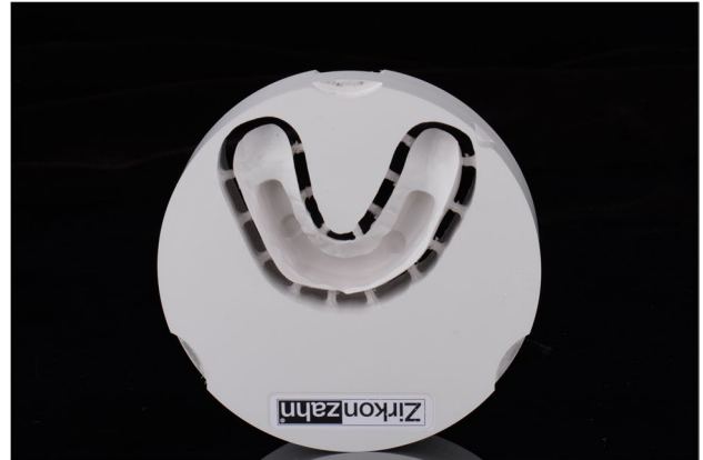
Fig. 64 CAD/CAM overdenture base material milled in ceramic reinforced PEEK
