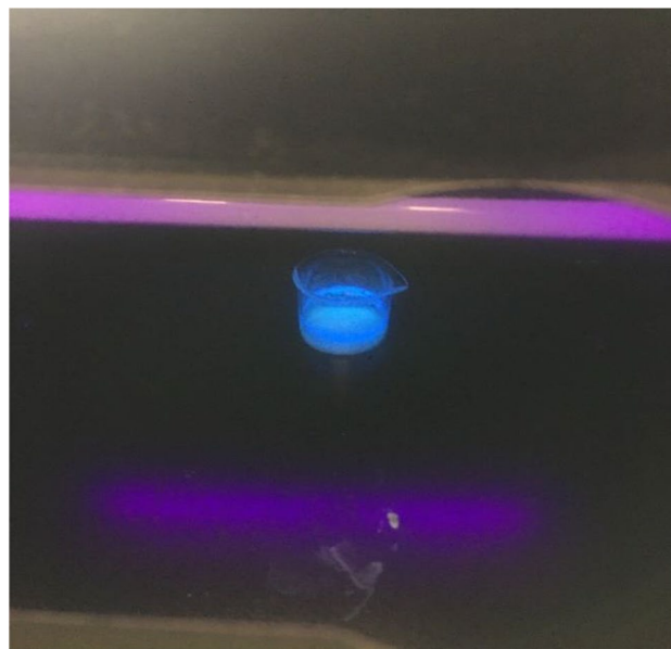
Fig. 2 Fluorescence observed from ZnS quantum dots when placed in the UV chamber
