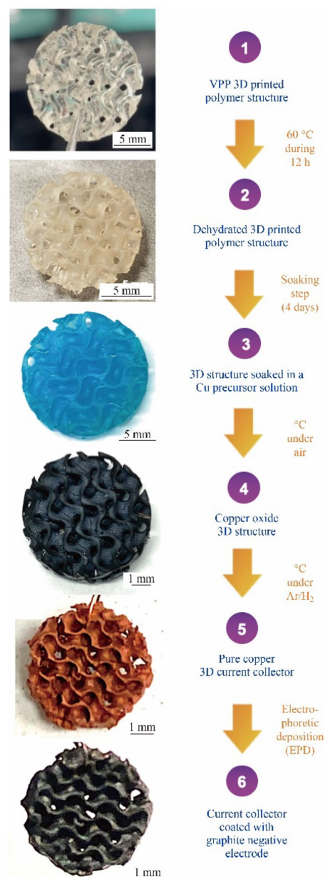
Fig. 1 Optical images of the fabrication steps leading to a negative electrode coated onto a VPP 3D printed current collector
