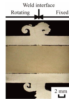
Fig. 9 Cross-section of weld interface region of joint using a CP-W core bar with diameter of 7.95 mm
