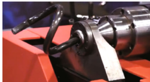
(d) Technology 4: bending by pressing pipes through a die
