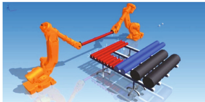
(e) Technology 5: bending by applying torque at both ends of a pipe (robot bending)
