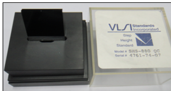
Fig. 1 Digital off-axis hologram recording setup based on Michelson interference and the sample for the height calibration (a Sketch map of the digital off-axis hologram recording setup based on Michelson interference, b–c Photo of the setup including the main optical path system and its platform, d Photo of the quartz step height standard (VLSI SHS-880QC))
