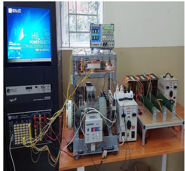
Fig. 15 The OPAL-RT system and experimental TIM model
