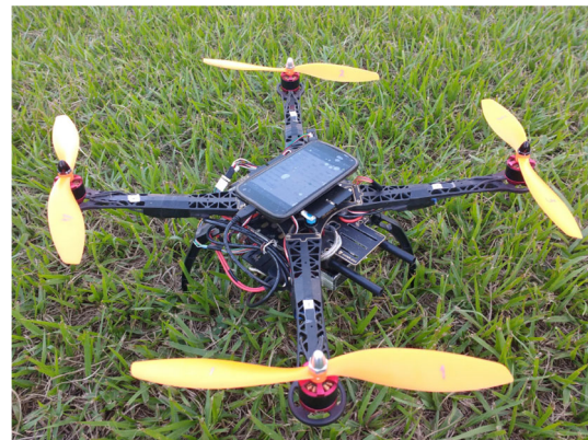
Fig. 9 Quadcopter used in [101] with an on-board smartphone as flight controller. Picture reprinted from [101]
