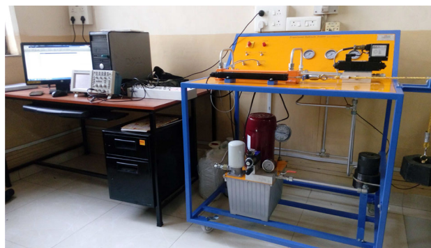
Fig. 7 Experimental set up of electro-hydraulic servo system
