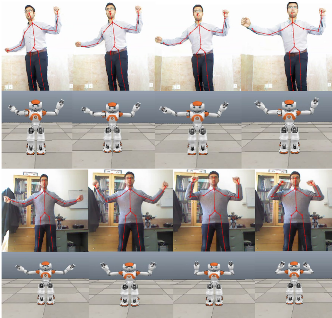
Fig. 8 System simulation in V-rep, Nao robot imitates human body movement
