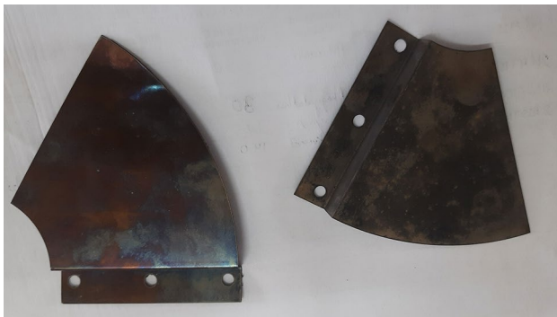
Fig. 4 Heat treated 75° steel foil and 45° copper foil of 0.4 mm thickness
