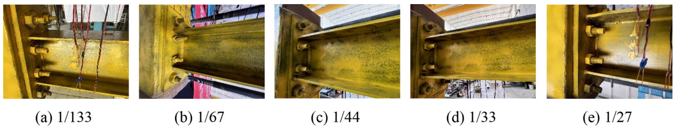
Fig. 15 The failure mode of steel beam joints under different horizontal drifts of the KJ-W
