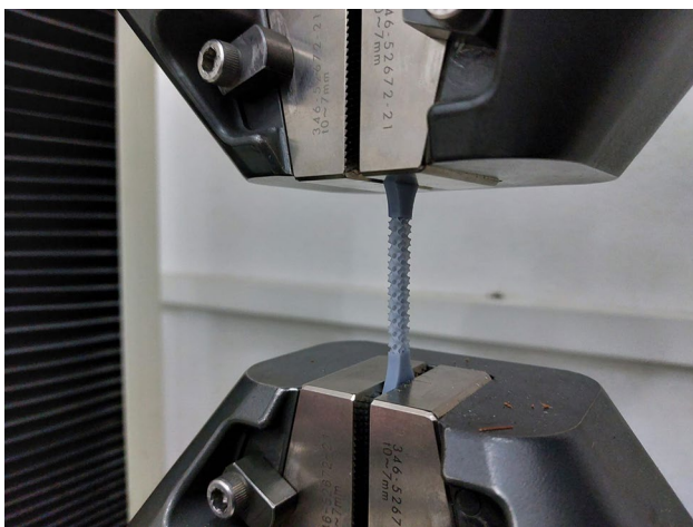
Fig. 4 A tensile test sample being tested
