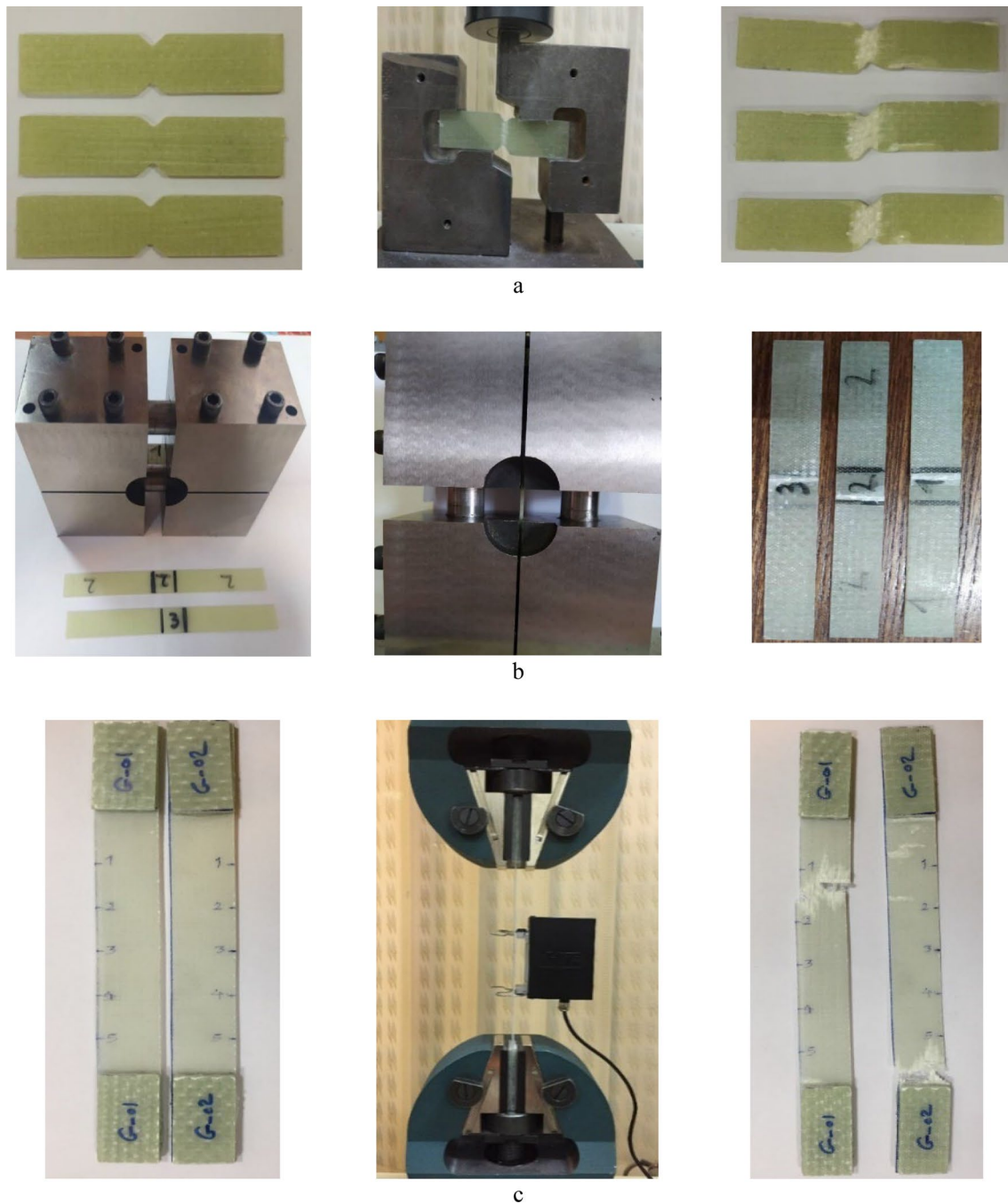
Fig. 5 The facesheet laminate samples under (a) shear test, (b) compression test and (c) tensile test
