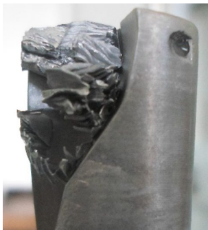
Fig. 8 Chips accumulated in the 4De U drill after drilling
