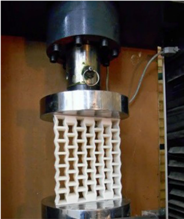
Fig. 6 The re-entrant auxetics structure under quasi-static loading
