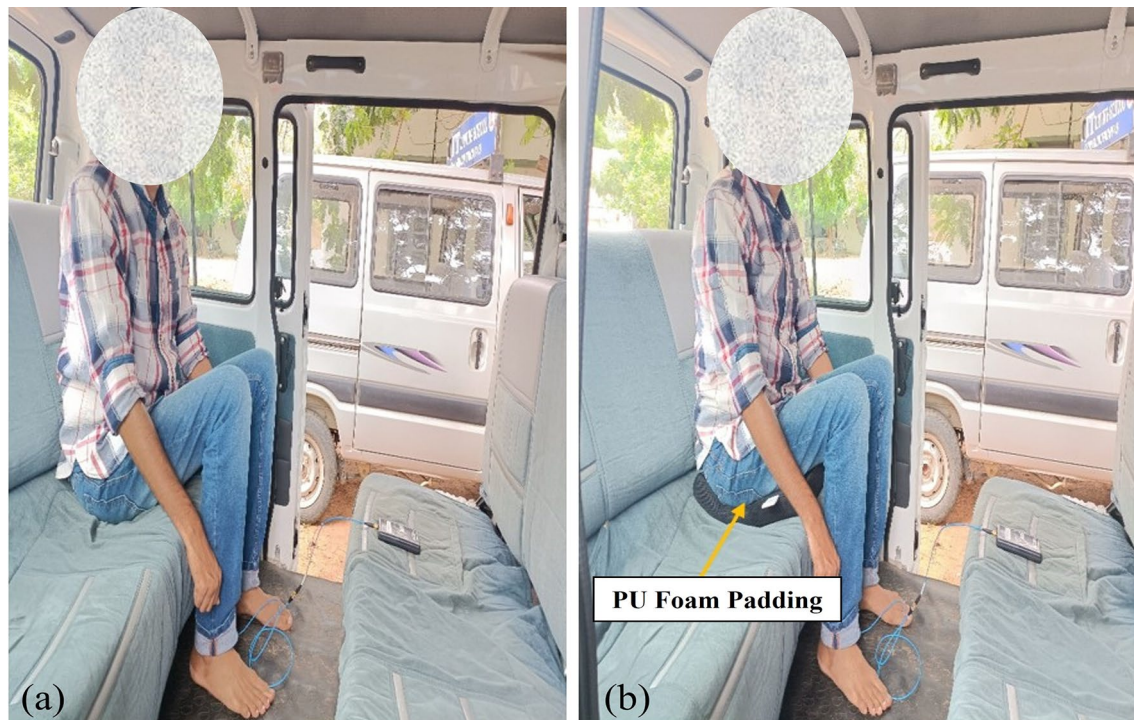
Fig. 2 a A triaxial accelerometer sensor installed on the seat without padding, b A triaxial accelerometer sensor installed on the seat with padding
