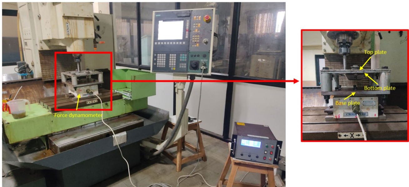
Fig. 4 Holding fixture on machine bed
