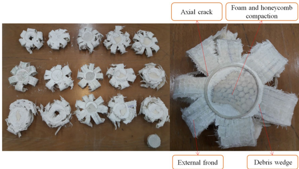
Fig. 14 Deformation mode of foam/honeycomb-filled tubes (Group 4)
