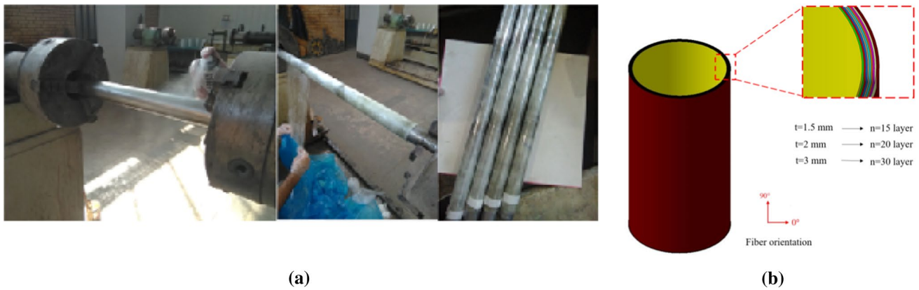
Fig. 5 a Preparation of the cylindrical composite tube, b The stacking scheme of the composite tubes with different thicknesses
