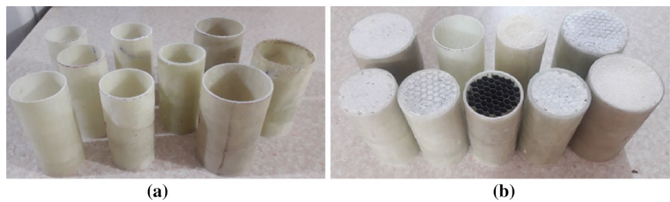
Fig. 5 a Preparation of the cylindrical composite tube, b The stacking scheme of the composite tubes with different thicknesses
