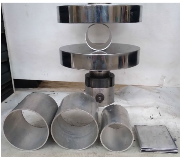
Fig. 5 How to place the samples between the jaws of the device
